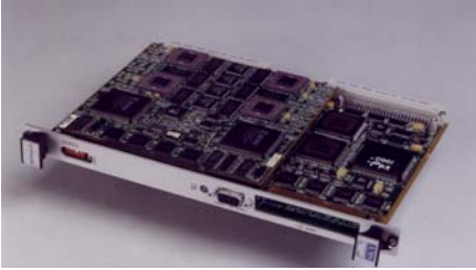
(Caption: The SKY Computers Merlin multicomputer is a COTS product build from the off-the-shelf MPC7400 microprocessors.)
